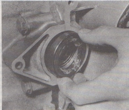
17.7 Locate a new oil seal
